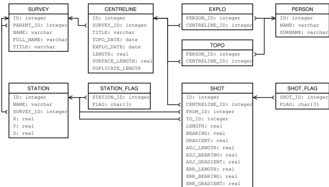
Table and column names are self-explaining; for undefined or non-existing values `NULL` is used. `FLAG` in `SHOT_FLAG` table is `dpl` or `srf` for duplicated or surface shots; in `STATION_FLAG` table `ent`, `con`, `fix`, `spr`, `sin`, `dol`, `dig`, `air`, `ove`, `arc` for stations with entrance, continuation, fixed, spring, sink, doline, dig, air-draught, overhang or arch attributes, respectively.
