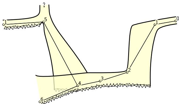
The only thing that is missing is connection line between stations 1 in these two branches. Therion does not automatically generate these lines because their shape usually depends on particular map.
