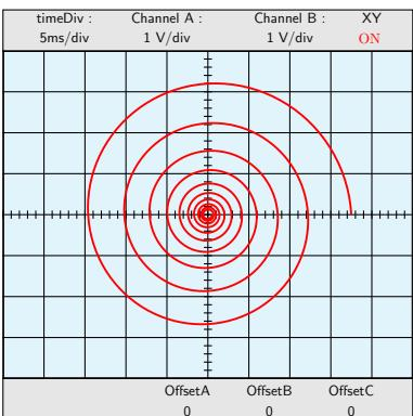
A damped LISSAJOUS diagram
