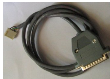
Figure 3.1: PC Parallel port cable for Serial loading of program memory.
