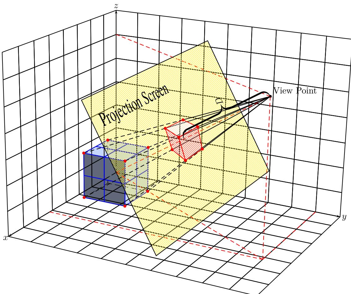
The coordinates of the object, in this case the bluish cube, are setup in the axes of coordinates  $Oxyz$ . The coordinates of the view point ( $V$ ), are setup in the same axes of coordinates, either in spherical
