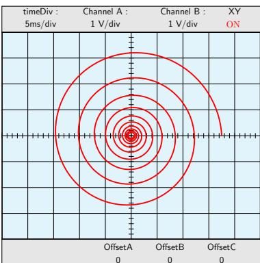
A damped LISSAJOUS diagram
